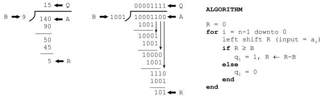
• An iterative architecture is depicted in the figure for *A* with 6 bits and *B* with 4 bits. The register *R* stores the remainder. A division operation is started when *E* = 1 (where *A* and *B* values are captured). Then, at every clock cycle, we either: i) shift in the next bit of *A*, or ii) shift in the next bit of *A* and subtract *B*. The signal *done* is asserted to indicate that the operation has been completed and the result appears in *Q* and *R*.
